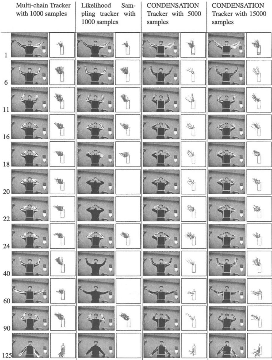
Fig. 3. Applying four tracking algorithms to a sample sequence. For each frame a set of four random pose samples were drawn from estimator posterior distribution and the corresponding skeletons was rendered (frontal view overlayed on the frame and side view next to it). Errors in feature detection caused likelihood-sampling tracker to fail on some of the frames (no samples were produced)
